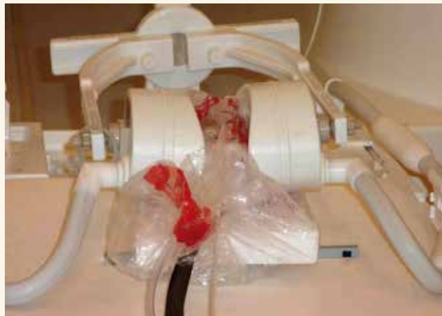
The hatching chick lies between the receiver coils normally used for human temporomandibular joints.
